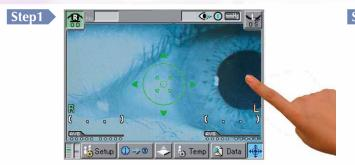
Simply touch the pupil center shown on the screen to roughly align the eye center with the center of the screen.
