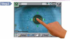
Lightly press the center of the screen to move the measuring head toward the patient. The Auto Alignment and Auto Shot functions will then quickly complete measurement.
